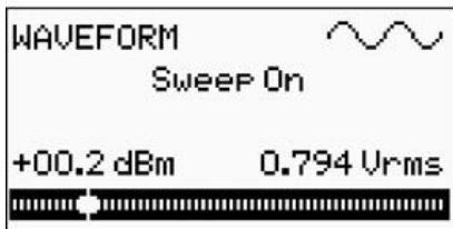
Waveform screen if Sweep is on. (inverse)
